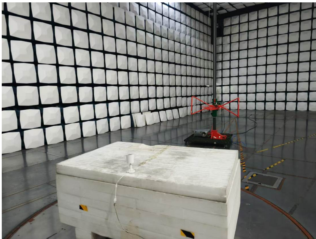
Radiated Emissions Below 1GHz rear View-Test Mode 1
