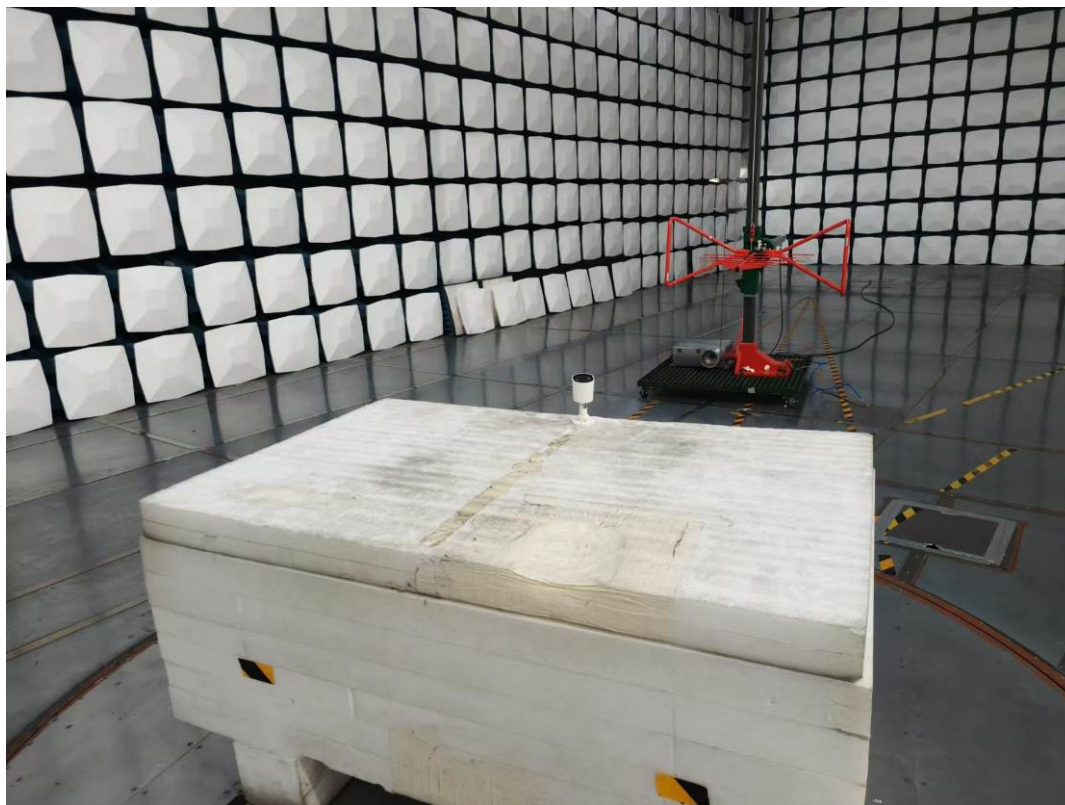
Radiated Emissions Below 1GHz rear View-Test Mode 2
