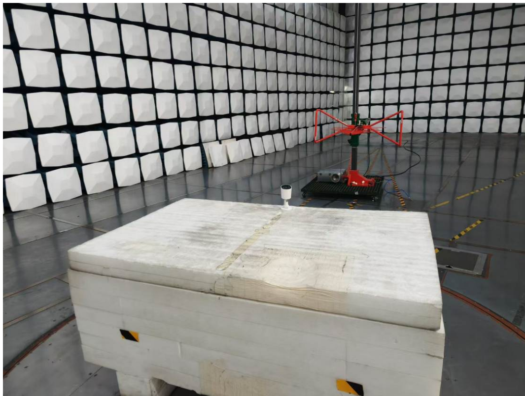
Radiated Emissions Below 1GHz rear View-Test Mode 1
