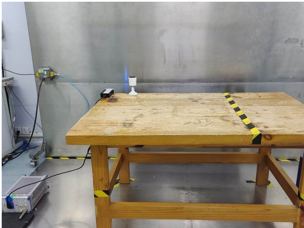
ISN Conducted emissions side View-Test Mode 2
