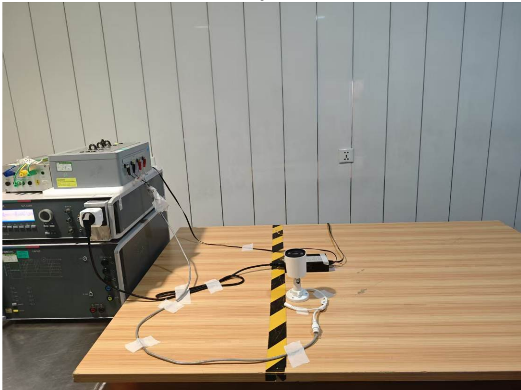
RJ45 Port Test Setup Photo Test Mode 2
