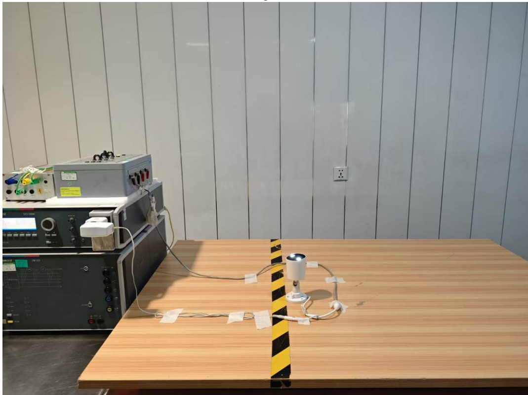
RJ45 Port Test Setup Photo Test Mode 1
