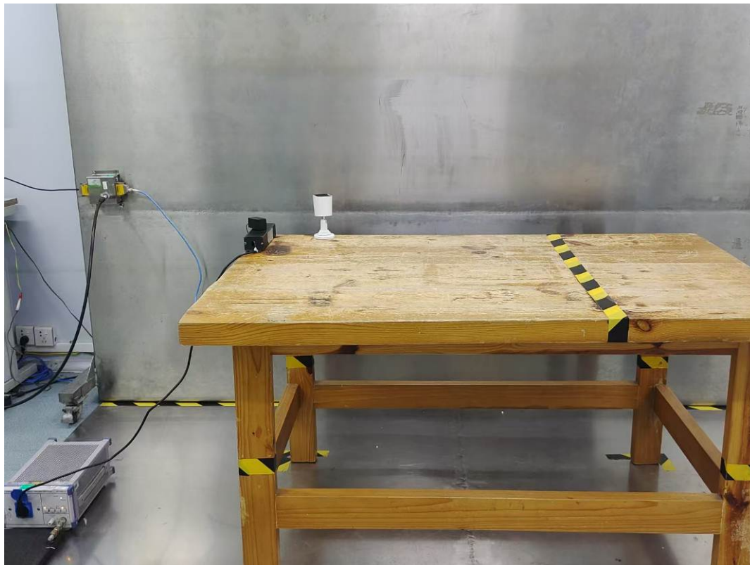
ISN Conducted emissions side View-Test Mode 1
