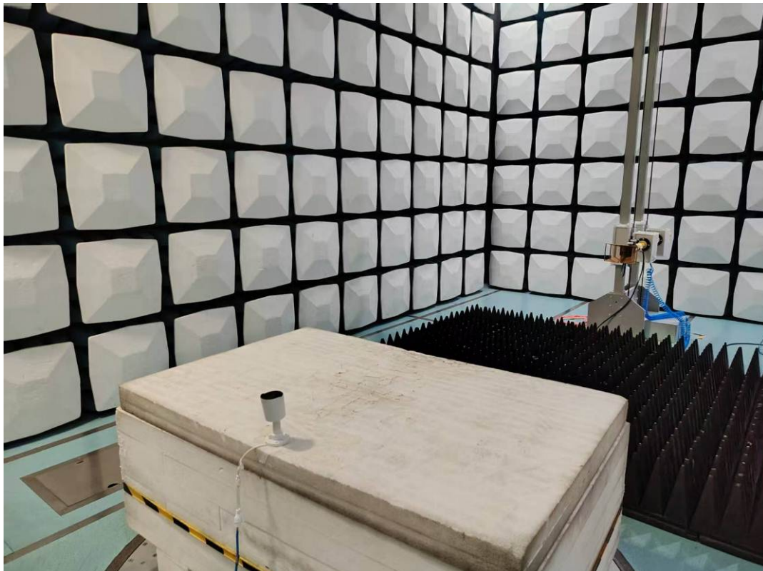
Radiated Emissions Above 1GHz rear View-Test Mode 2
