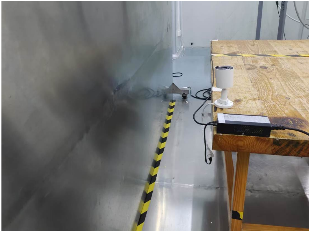
Conducted emissions side View-Test Mode 2
