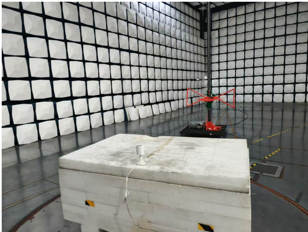
Radiated Emissions Below 1GHz rear View-Test Mode 2
